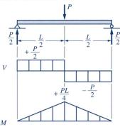
**2.** Simple beam with a concentrated load at any point
